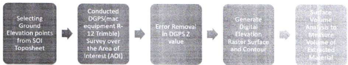
Figure 2: Methodology for calculation volume of Extracted Material
